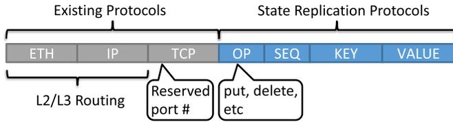
Fig. 9. Format of the state replication packets.
